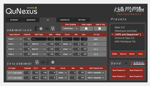
Here you can choose how the QuNexus keys send and receive CV (Control Voltage) QuNexus has 4 possible CV outputs and 2 possible CV inputs (see the CV chapter for the hardware specs).
