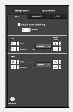
how hard the sensor was struck, and a continuous CC# value corresponding to the pressure exerted on the sensor. Setting a numerical value in the number box will override the default behavior and output just that value.
