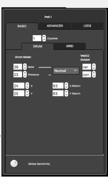
To the right of the toggle menu are number boxes for **setting Velocity and Pressure values**. By default these boxes are set to "var" for "Variable Velocity" and "con" for "Continuous Pressure". In default mode the sensor will send out a Velocity value related to how hard the pad was struck, and a continuous CC# value corresponding to the pressure exerted on the sensor. Setting a numerical value in the number box will override the default behavior and output just that value.
