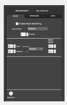
continuous CC# value corresponding to the pressure exerted on the sensor. Setting a numerical value in the number box will override the default behavior and output just that value.
