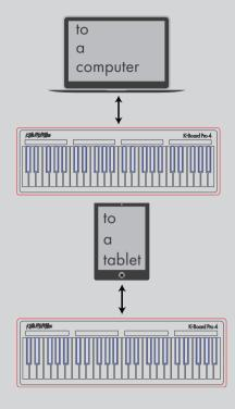
Use the provided Micro-USB cable to connect your K-Board to computers or tablets. Simply plug the micro end into the K-Board's USB port, and the other end into a USB port on the desired device.
