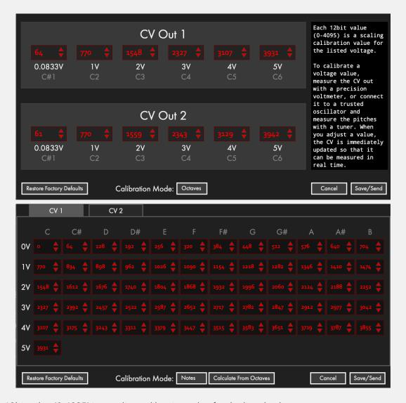
Each 12bit value (0-4095) is a scaling calibration value for the listed voltage.
