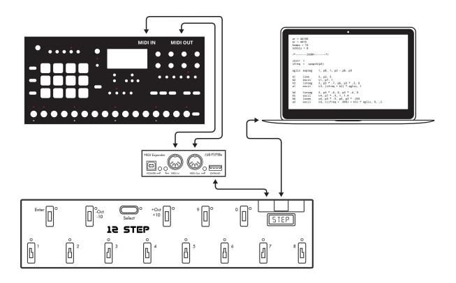
The 12 Step can be connected to both a computer and external MIDI hardware at the same time (KMI MIDI Expander required).
