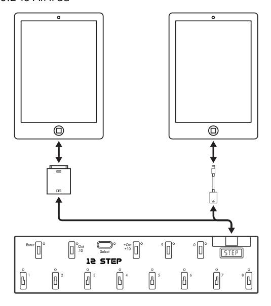
Connecting the 12 Step to an iPad is very similar to connecting to a computer, the only difference is that one more part is needed.
