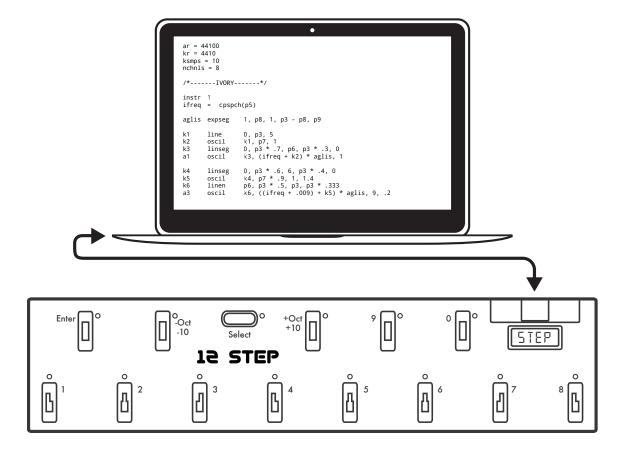
Connecting the 12 Step to a computer requires three things: a 12 Step, a computer, and a USB A to USB B cable (the "classic" USB cable). Simply plug the 12 Step's main USB port into a USB 2.0 (or greater) port on the computer. The 12 Step will receive power from the computer.
